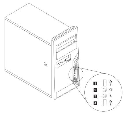
Figure 1. Front connector locations
